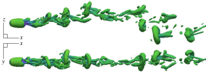
FIGURE 17. Wake observed in mode III ( Re = 1200 , m^* = 80 , l^* = 10 and U^* = 30 ) visualized with isosurface of Q = 0.001 . Flow from left to right.
