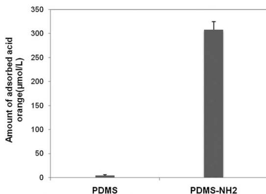
Fig. 3 Quantification of surface amine on native PDMS and PDMS-NH<sub>2</sub> by measuring the amount of adsorbed acid orange.
