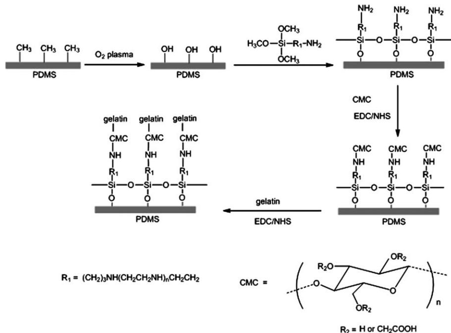
Fig. 2 Schematic illustration of the surface functionalization procedure.
