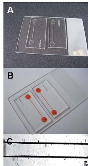
**Fig. 1** Photos of (A) a PDMS micro-bioreactor, (B) a food-dye filled micro-bioreactor device showing inlets, outlets and microchannels, (C) an enlarged bright field view of a microchannel, photo taken under an optical microscope (scale bar = 100  $\mu\text{m}$ ).
