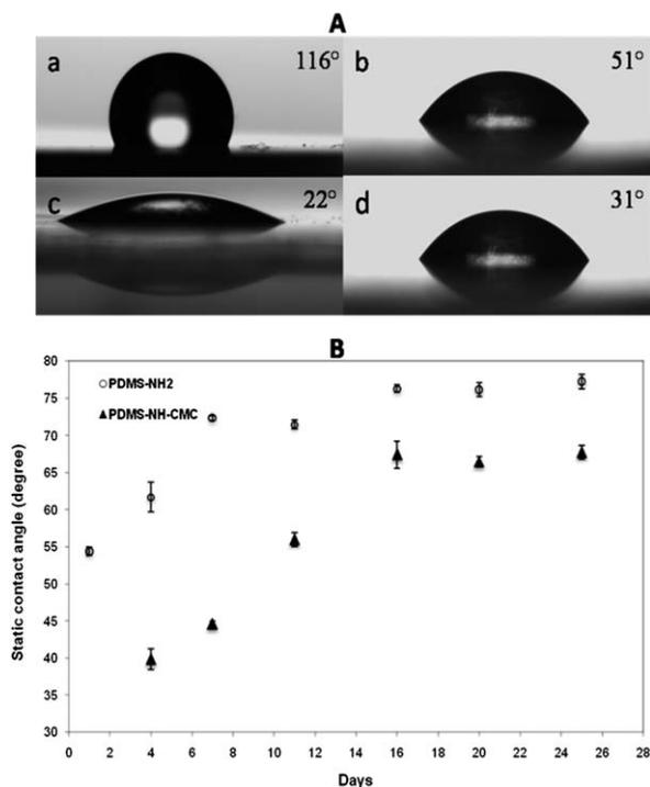
**Fig. 5** (A) Static water contact angle of (a) PDMS, (b) PDMS-NH<sub>2</sub>, (c) PDMS-NH-CMC, and (d) PDMS-NH-CMC-GEL substrates measured at day 1. (B) shows the variation of static contact angles of PDMS-NH<sub>2</sub> and PDMS-NH-CMC as a function of the storage time in air.
