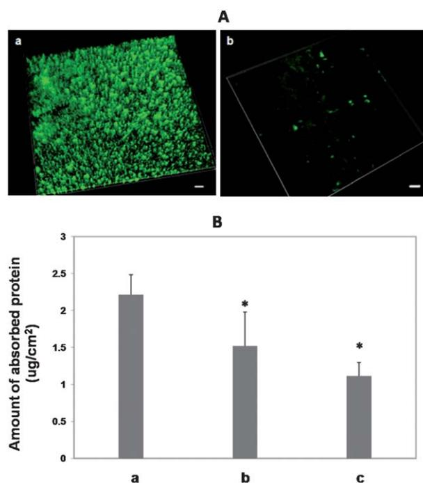
**Fig. 6** (A) Confocal microscopy images showing BSA-FITC adsorption on PDMS and PDMS-NH-CMC (scale bar = 100 μm). (B) shows the influence of surface modification on BSA adsorption on (a) PDMS, (b) PDMS-NH<sub>2</sub>, and (c) PDMS-NH-CMC substrates. Data are presented as average values ± standard deviation (\**p* < 0.05).
